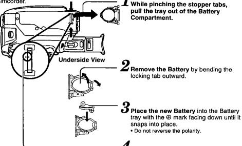
**Replace the Battery tray** so that the small triangle marks meet.
