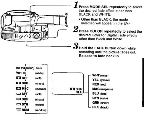
To create even more special effects, (other than BLACK, WHITE, and RANDOM modes), you may also partially fade the picture, and by pressing the MODE SEL button, freeze the fade function. Press FADE again to resume, or press
