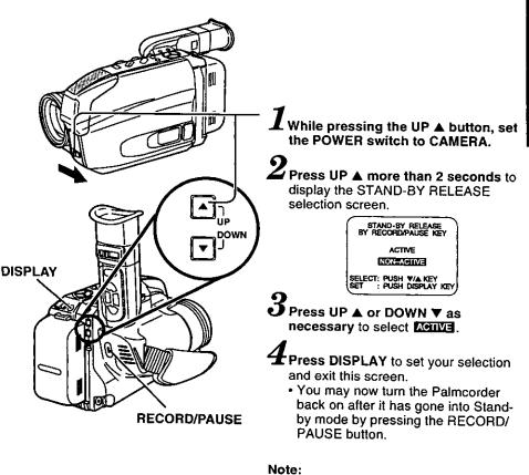
If **NON-ACTIVE** was selected in step 3 above, you must set the POWER switch to OFF and then to CAMERA to resume recording from Stand-by mode.
